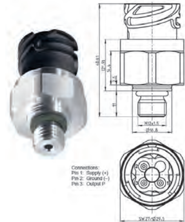
Electronic pressure sensor with voltage output
